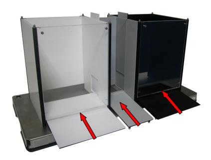
Figure 3. Placing the floors in the cage.
